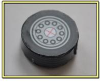
18. Glue the back wheel face 6 onto the other side of the wheel.
