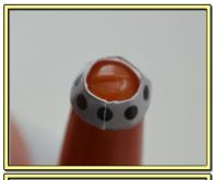
13. Forming part 3 is easy with the use of a suitable dome-shaped object such as the end of a tool handle.
