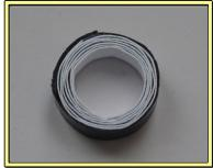
9. Put it into the inside of the cylinder and allow it to spring out to hold the wheel into a circle. Note: if the spiral is more than 2.5mm thick, cut some off it and recoil it.
